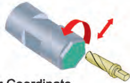
Polar Coordinate Interpolation (For C-axis)
