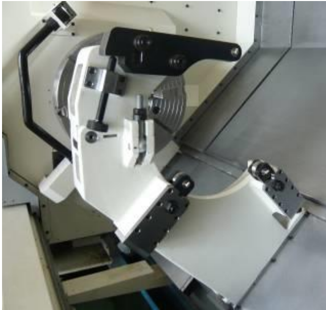
Manual steady rest clamping range 40~400mm
