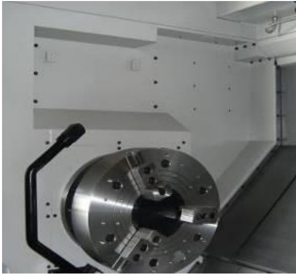
The concave spindle guard prevents any tool interference
